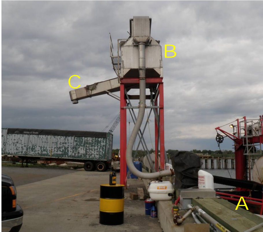
Figure 12. At this port herring are unloaded from the vessel, into tubes on the dock (A), up through another tube and into a dewatering box (B). Trucks drive under the end of the dewatering box (C) and fish are dumped into containers or the truck itself (not pictured).
